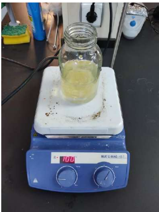
Figure 2.3 - IKA C MAG HS 7 magnetic stirrer and electronic scales
